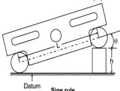
The angle formed between the upper surface of a sine bar and the surface plate (datum) =  $\sin \theta = \frac{H}{L}$
